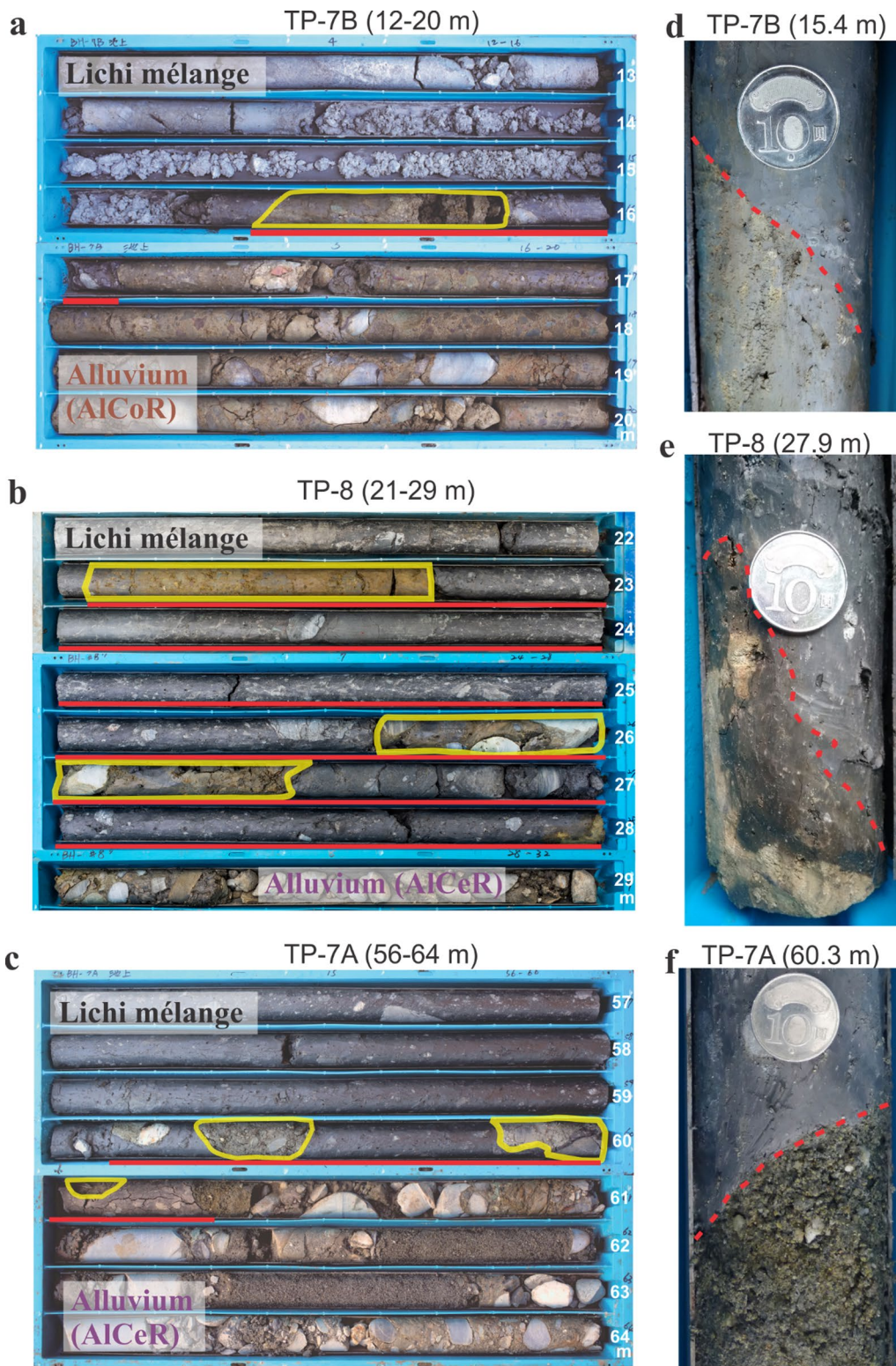
Fig. 7 Fault contacts/fault zones in the rock cores. Red lines highlight the mixed zone/fault zone between Lichi Mélange and alluvium deposit. Yellow polygons denote deformed alluvium deposits in the Lichi Mélange. a Rock core of TP-7B at depths of 12 to 20 m. b Rock core of TP-8 at depths of 21 to 29 m. c Rock core of TP-7A at depths of 56 to 64 m. d Fault contact between mud of Lichi Mélange (at right) and fine-grained sand of alluvium (at left) in TP-7B at depth of 15.4 m. e Fault contact between mud of Lichi Mélange (at right) and fine-grained sand of alluvium (at left) in TP-8 at depth of 27.9 m. f Fault contact between mud of Lichi Mélange (at left) and very coarse-grained sand of alluvium (at right) in TP-7A at depth of 60.3 m
